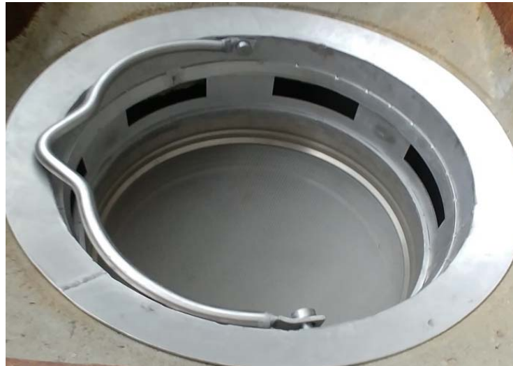
Picture 2: The sampling basket for drains developed by GKD allows a defined fractionation of particulate material in the fight against microplastics.
