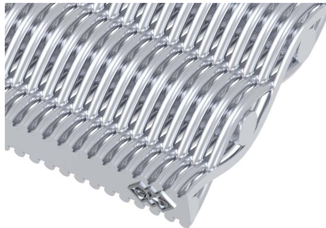
Picture 2: The special weave creates a slot-shaped pore geometry on the mesh surface, whose openings are smaller than the pores inside the mesh.
