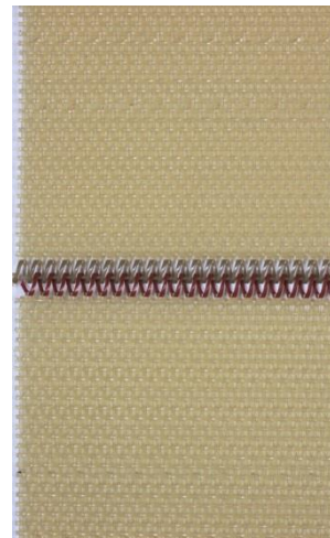
Picture 4: PPS belt for ADL processes with woven spiral seam.
